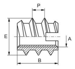
Female thread A = M8Length B = 20Male thread E = 13.0Min hole depth = 23
